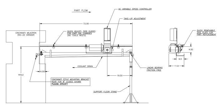
**APPLICATION:** Convey Steel Tubes to the workrest of a CINCINNATI Model 340-20 Centerless Grinder.
