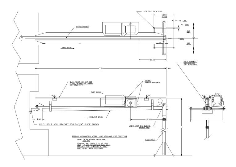
**APPLICATION:** Convey Bearing Cups away from the workrest of a CINCINNATI GRINDING CL-500
