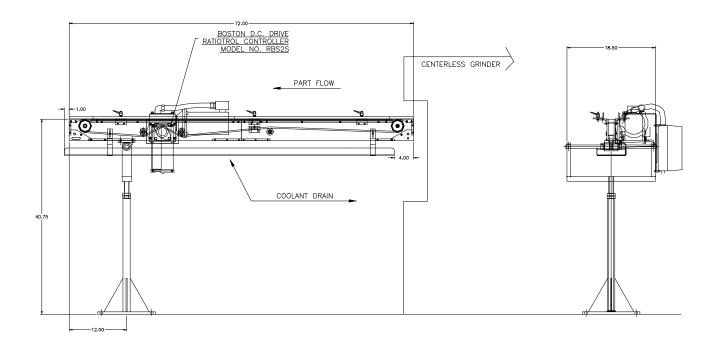
**APPLICATION:** Convey Compressor Pistons away from the workrest of a CINCINNATI Centerless Grinder.
