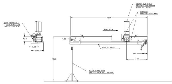
**APPLICATION:** Convey Shafts to the workrest of a LANDIS Centerless Grinder.
