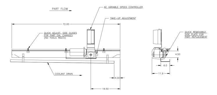
**APPLICATION:** Convey parts to the workrest of a CINCINNATI Centerless Grinder.
