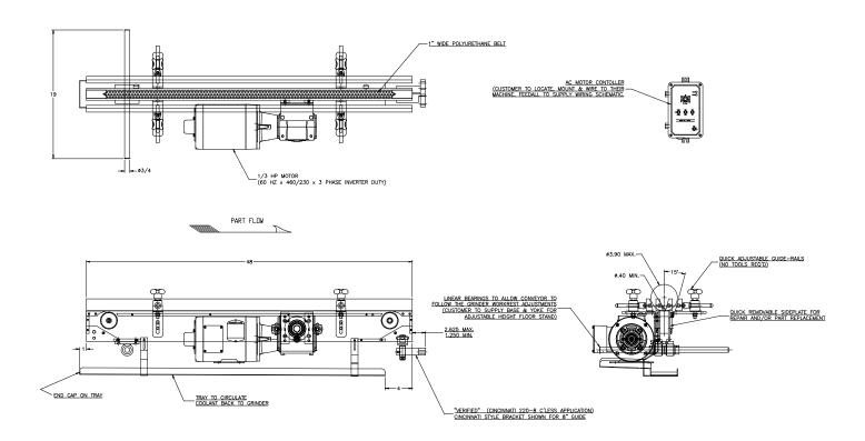
**APPLICATION:** Convey Ceramic Rounds to the workrest of a CINCINNATI Model 220-8 Centerless Grinder.
