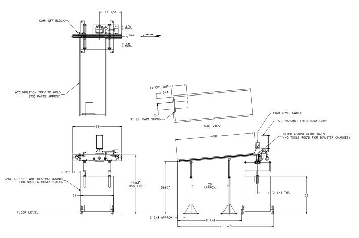
**APPLICATION:** Convey Agitator Shafts from a Centerless Grinder to a cam-off accumulation ramp.
