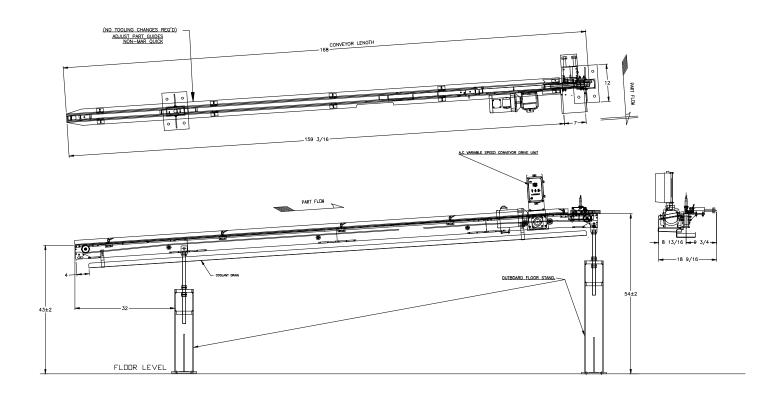
**APPLICATION:** Convey Steel Bushings from Acme Centerless Wire Brush to End Finisher.
