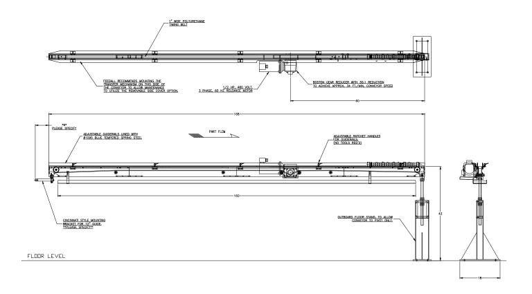
**APPLICATION:** Convey Cam Shafts to the workrest of a CINCINNATI Centerless Brush Machine.
