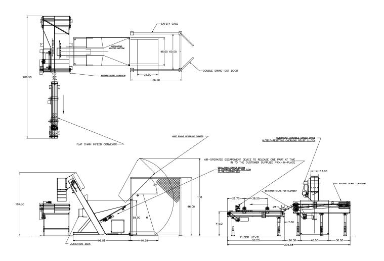
**APPLICATION:** Feed from a tub dumper into a floor mounted hopper. The Universal Joint Spiders will be
