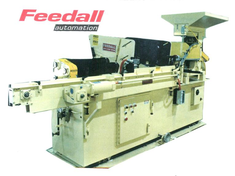
FEED FROM A MANUALLY LOADED MAGAZINE, STEEL BARS AND TUBES, 3/8 TO 1 3/8 DIA. X 3 1/2 TO 44" LG. AND FEED FROM A HOPPER LOADED BOWL STEEL PINS 3/8 TO 3/4 DIA. X 1 3/4 TO 3 1/2 LG. TO A CENTERLESS GRINDER AT 42 3/4" ABOVE THE FLOOR. FEED RATES OF 50 TO 150" PER. MIN. DWG. PD 8072R 1
