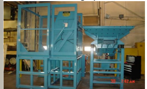
Dumper w/Vibratory Metering Hopper
