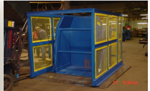
Hydraulic Tub Dumper
