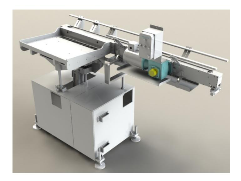
**APPLICATION:** Feed from a manually loaded, single row magazine Crosshead Pins. Pins will be
