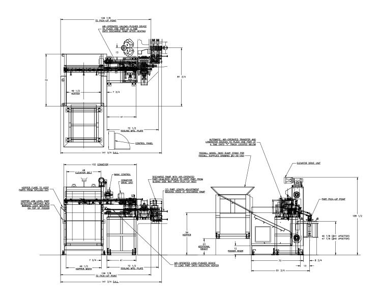
**APPLICATION:** Feed from a random loaded floor mounted hopper. The Saw-Cut Steel Billets will be elevated
