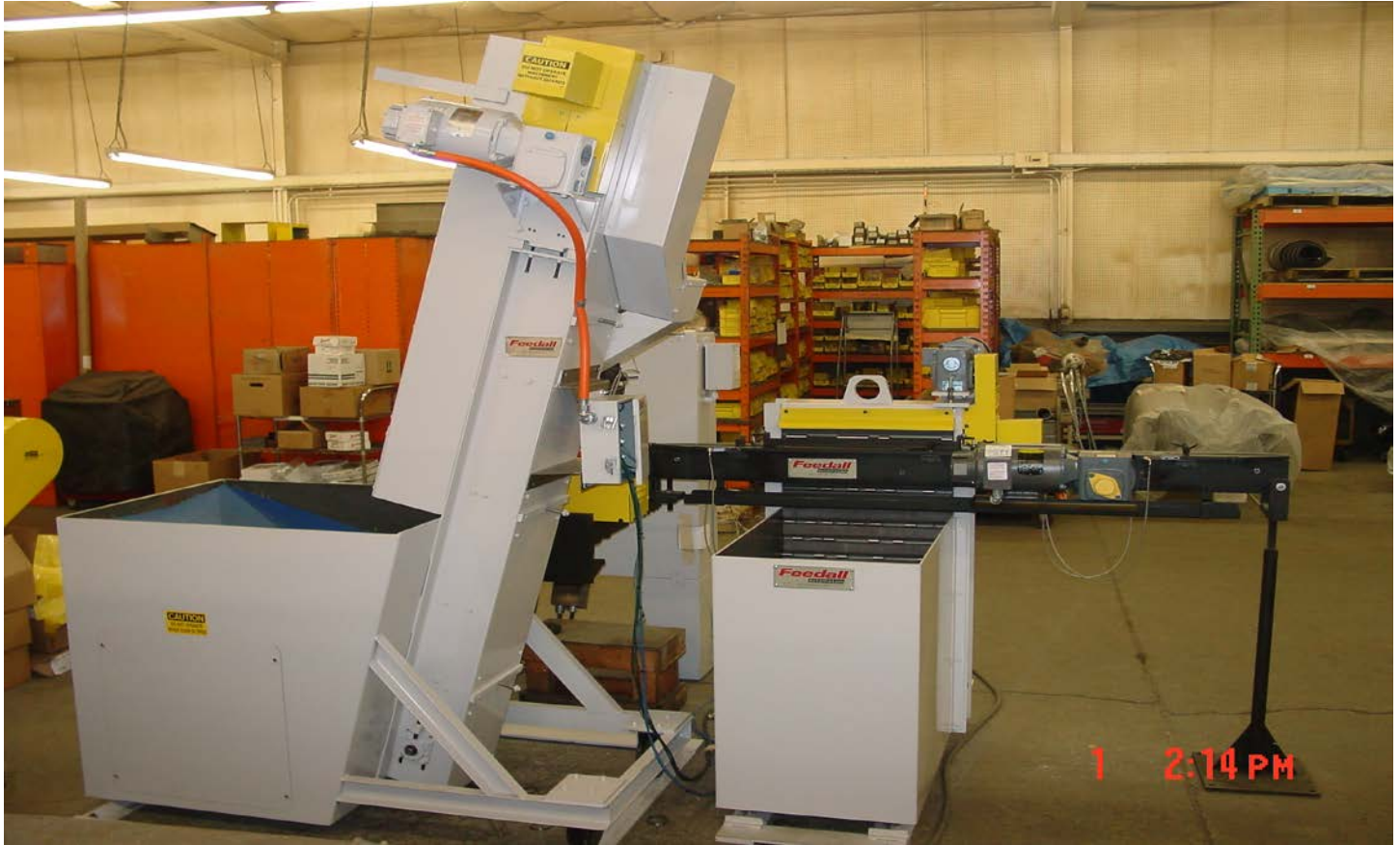
FEEDALL Model 2400-D w/Model 2000 to feed Piston Rings and Valve Guides into Centerless Grinder
